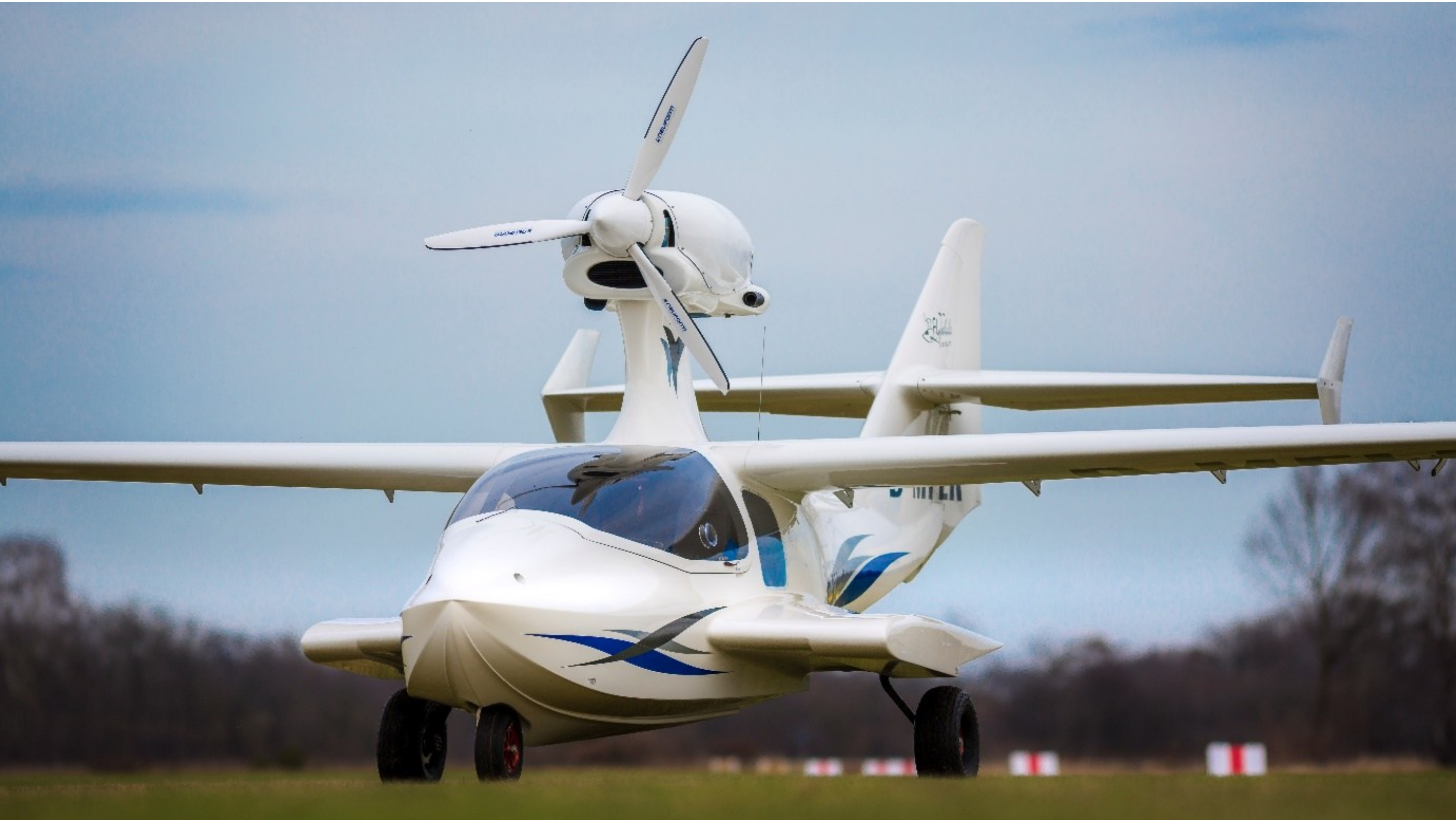
Figure 1: The Flywhale FW650 (Uniplanes GmbH), today Dornier Seawings DS-2C, is a German two-seat amphibious sports aircraft in the 650-kg-class. More: Bachelor Thesis, Gmelin 2022, https://doi.org/10.5281/zenodo.15618552 .
